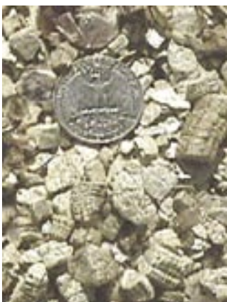
Figure 4. Vermiculite that has been "popped" by heating to remove moisture
